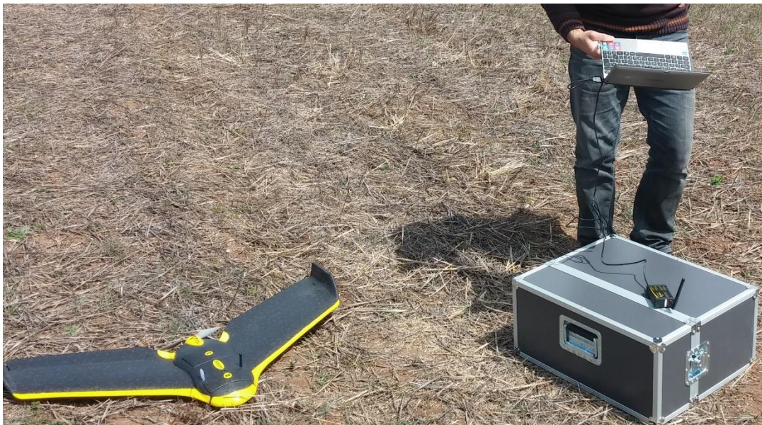
Figure 3.5. UAV and ground control station
