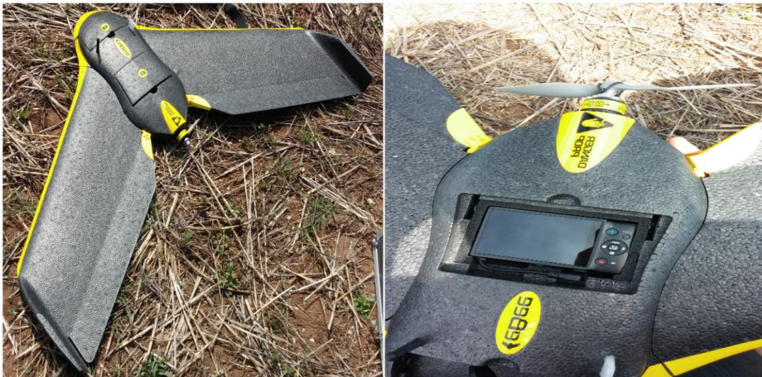
Figure 3.2. eBee UAV platform with the supplied camera.
