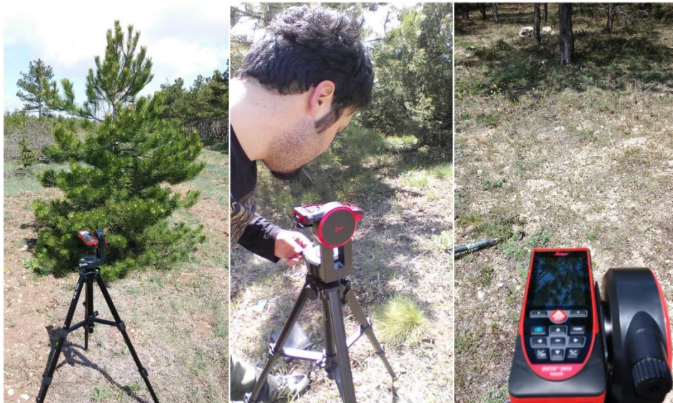
Figure 3.6. Ground measurements were taken with a laser distance meter platform
