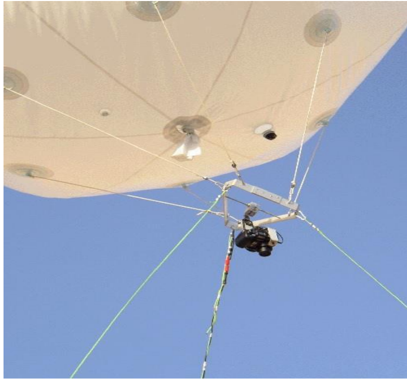
Figure 1.1. The camera platform below the balloon with the balanced holder of the camera and the ropes [12]
