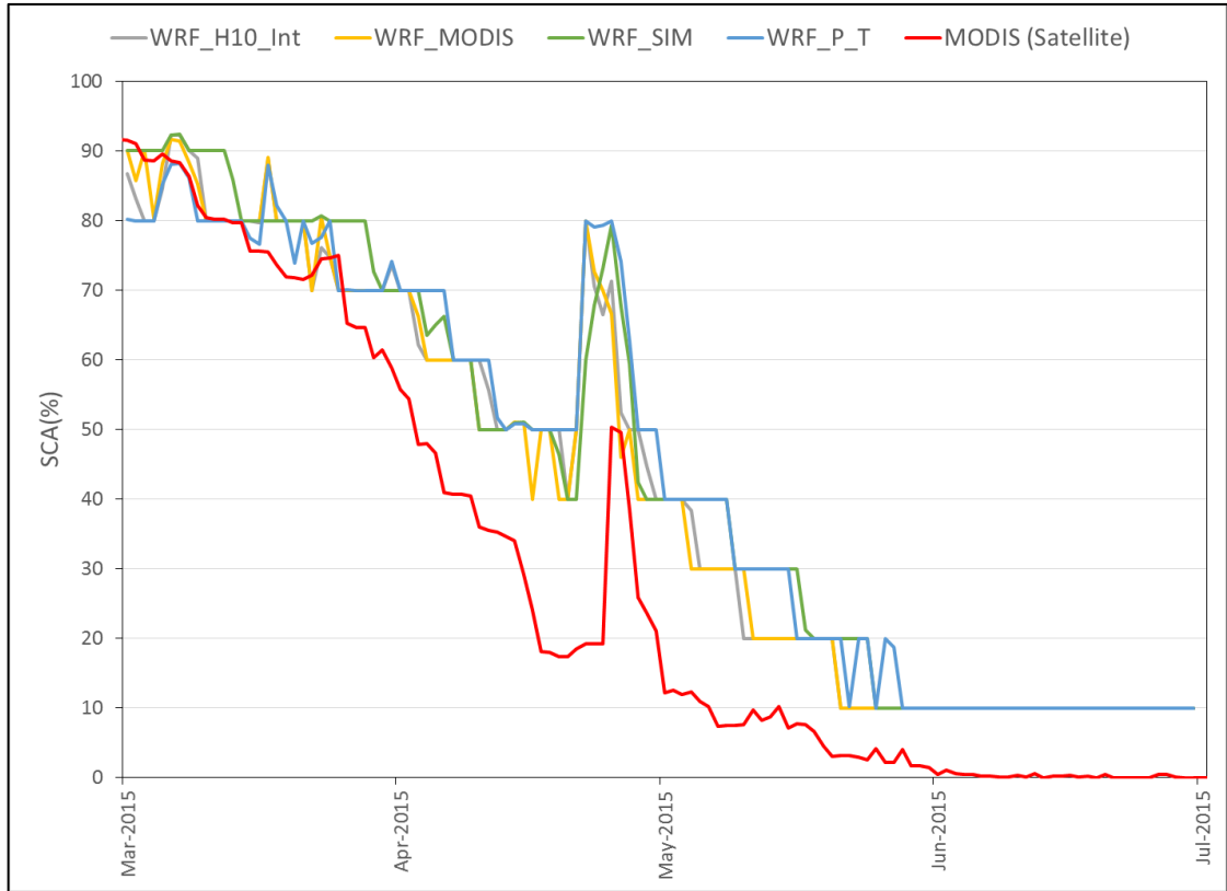
Figure 5.28. Comparison of SCA in Karasu Basin with WRF data for 2015 water year.
