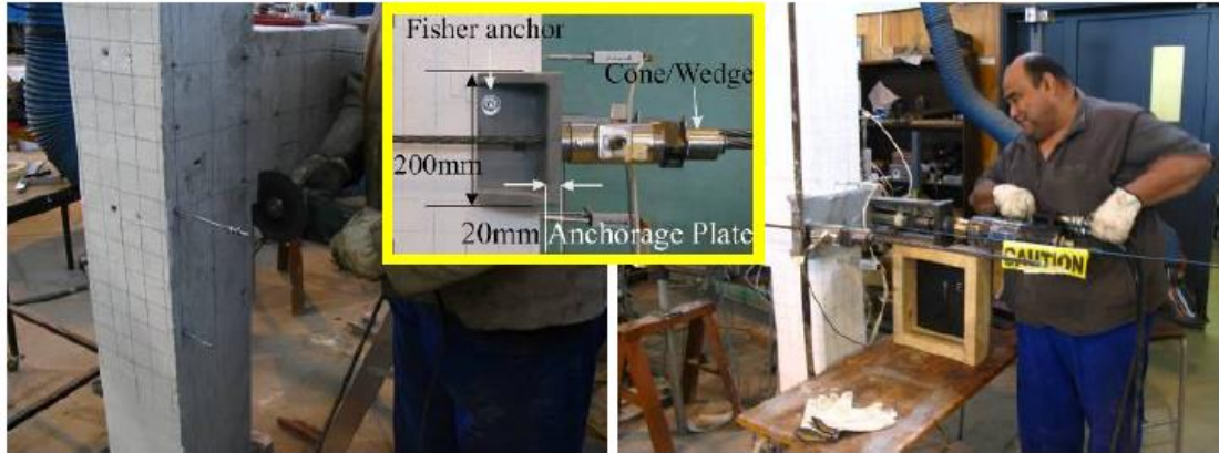
Figure 3.21. Beam weakening and application of post-tension [36]
