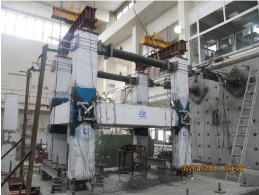
Figure 3.17. CFRPs retrofitted specimen [31]
