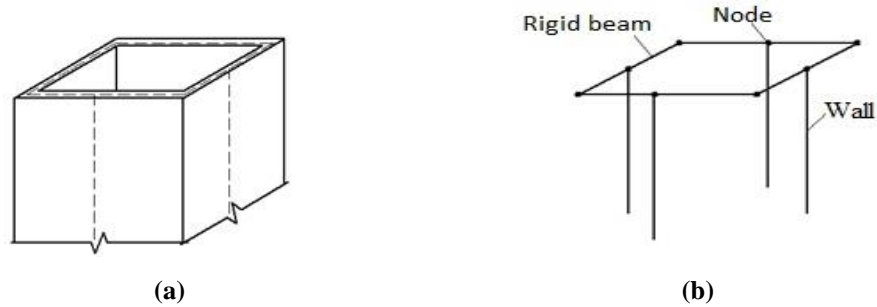
Figure 4.3. Shear wall model a) 3-D view, b) mathematical model
