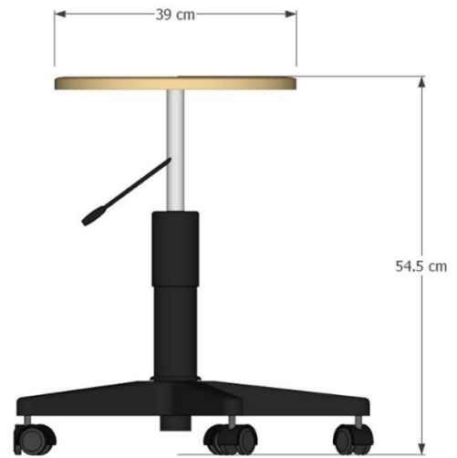
Figure 6.27. METU, Architecture design studio's stool dimensions with maximum adjusted seat height.
