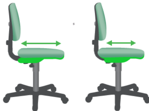
Figure 4.4. A seat depth (Adjustable).
