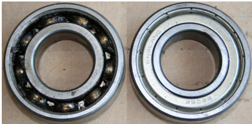
Figure 3.3. Faulty and unused bearings
