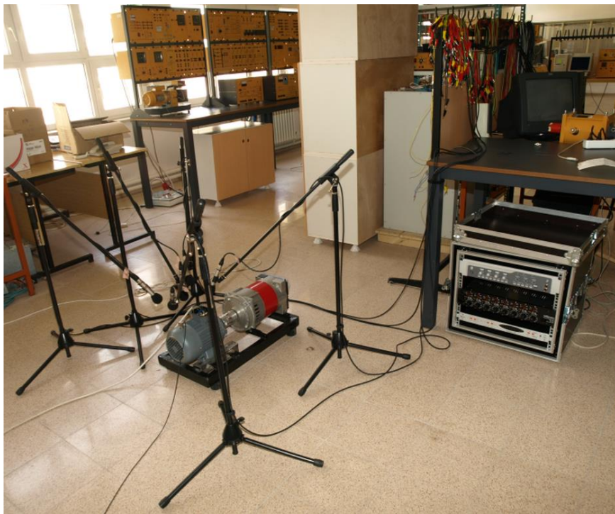
Figure 3.6. The placement of the microphones over test rig
