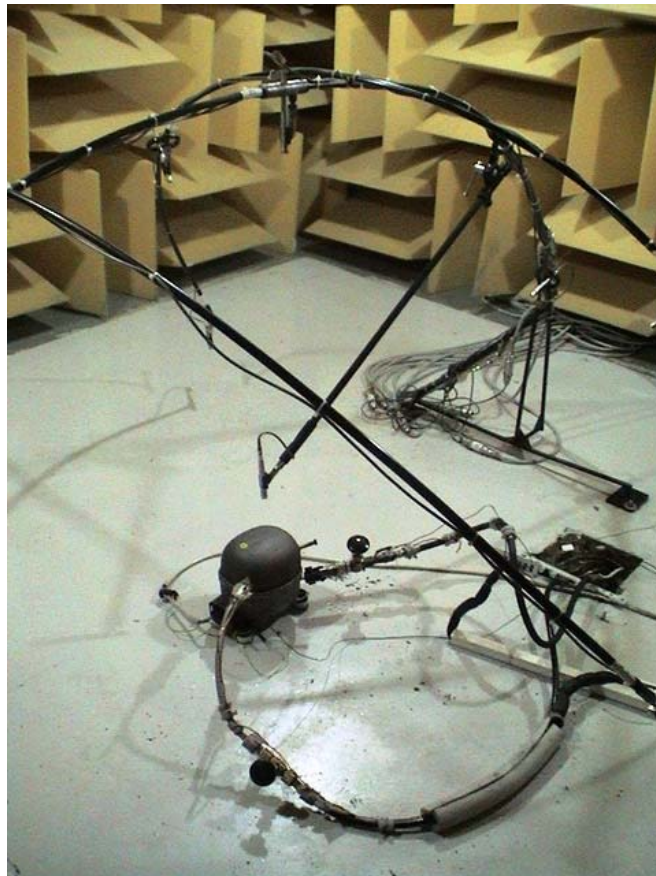
Figure 10: A Compressor in the Test Room (date taken: 20-April-2006)
