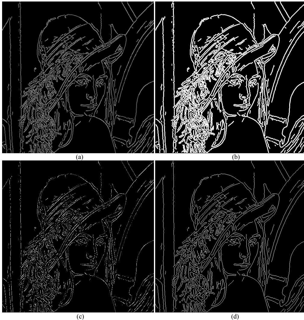
Figure 3.3: (a) Canny’s BEM smoothed by a Gaussian kernel with \sigma = 0.50 , (b) Thresholded smoothed edge map: the extended edge areas, (c) Anchors extracted from Canny’s BEM, (d) Final edge segments after SR. Edge segments shorter than 8 pixels have been eliminated.
