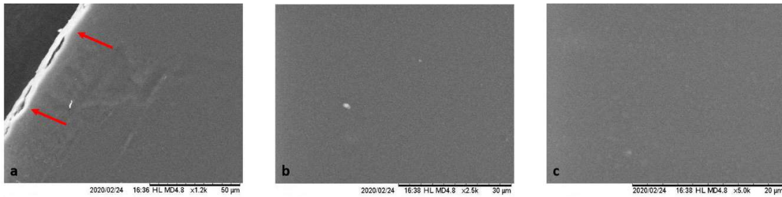
Figure 5.12. SEM images of D1 film at different magnifications a: 1.2 K X (The red arrows show the edge of the film), b: 2.5 K X, c: 5.0 K X
