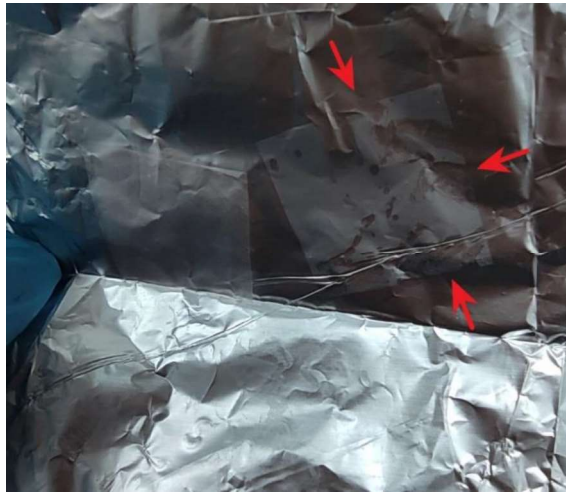
Figure 5.14. Part of the film stuck on the aluminum foil because of moisture uptake
