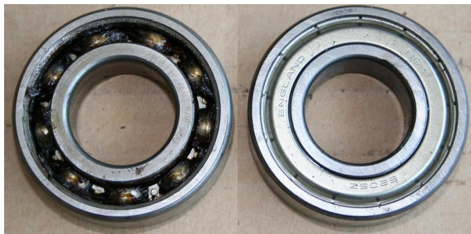
Figure 2.2. Faulty and unused bearings respectively
