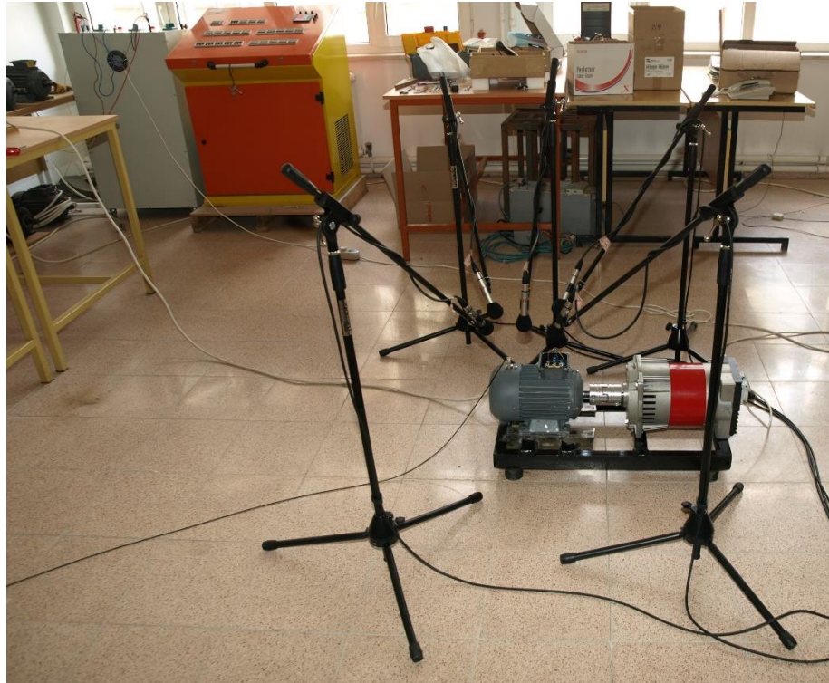
Figure 2.6. Experimental Setup for vibration and acoustic data
