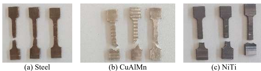
Figure 3.13. Tested dog-bone shaped specimens of upgrading materials
