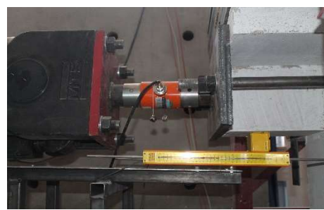
(b) Close view of MTS-frame connection
