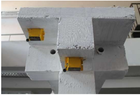
(a) Accelerometers at the front end
