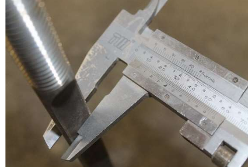
(d) Measuring of section height before the test
