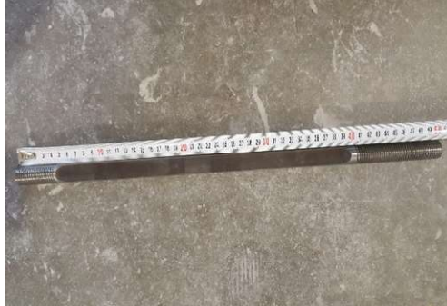
(e) Length of the NiTi bar after the test
