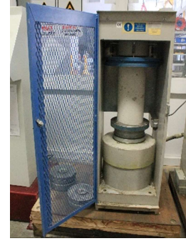
(c) Uniaxial compression test
