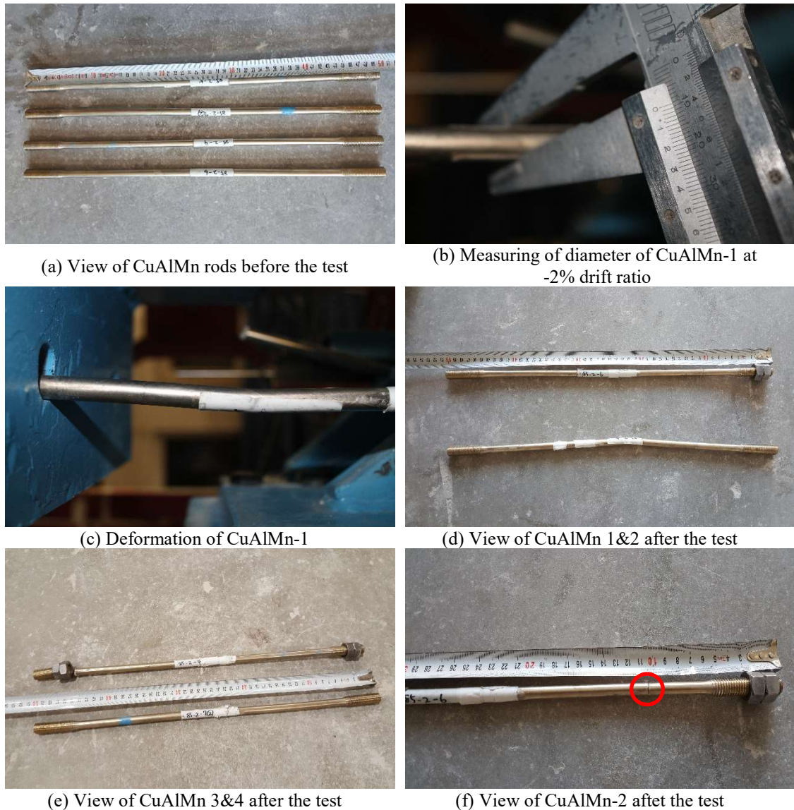
Figure 4.15. Failure pattern of CuAlMn rods during and after the test
