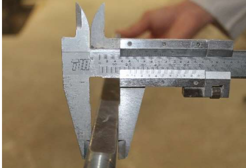
(c) Measuring of section width before the test
