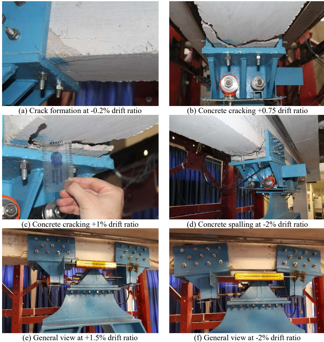
Figure 4.22. Failure pattern of U-shaped plates during cyclic loading
