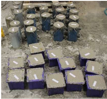
(a) Cylindrical and cubic specimens after casting
