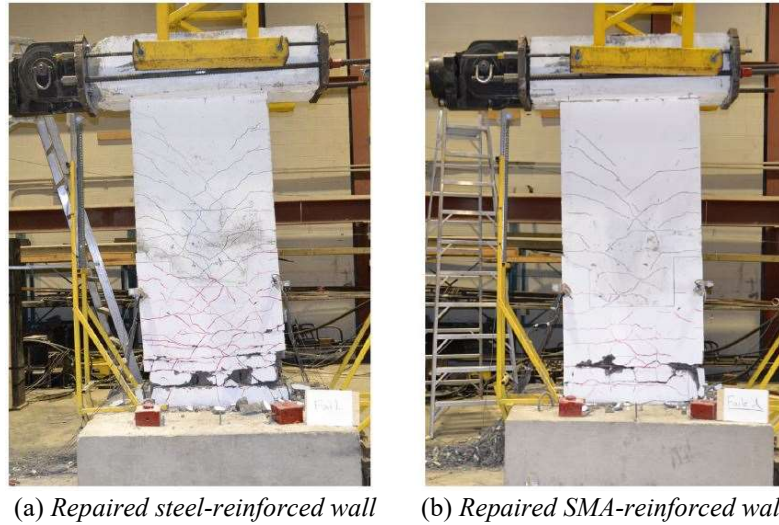
Figure 2.10. Condition of walls at the end of testing (Cortés-Puentes et al. 2018)
