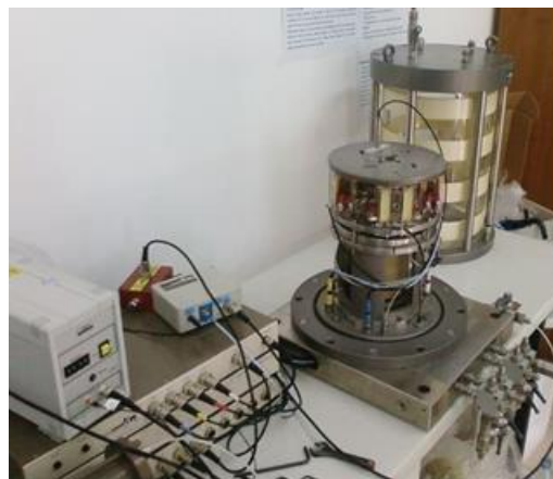
Fig. 1: GDS resonant column test device.
