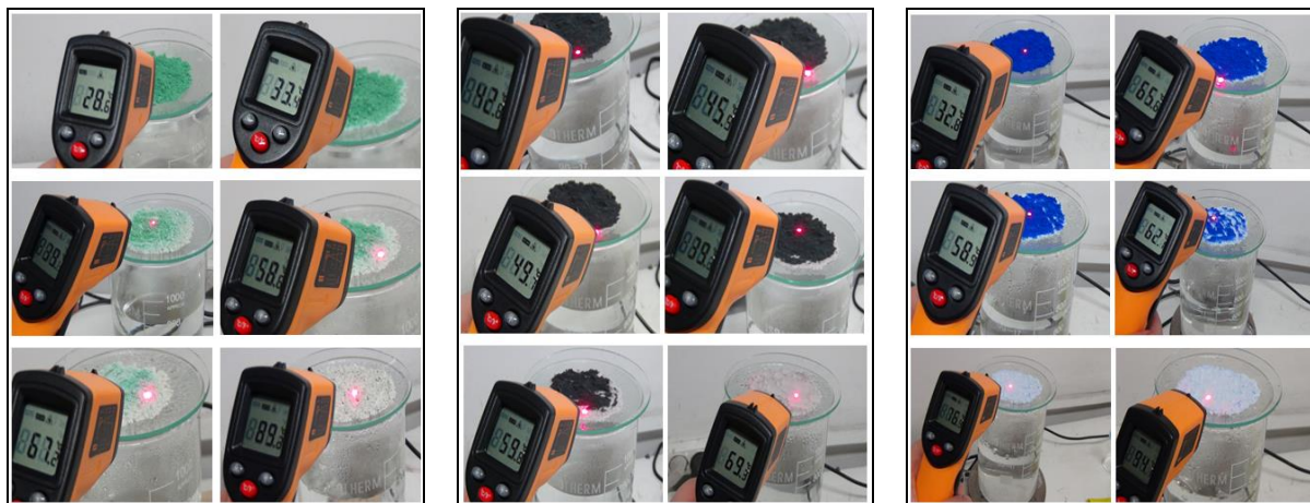
Figure 4. Color change of thermochromic pigments with increasing temperature
