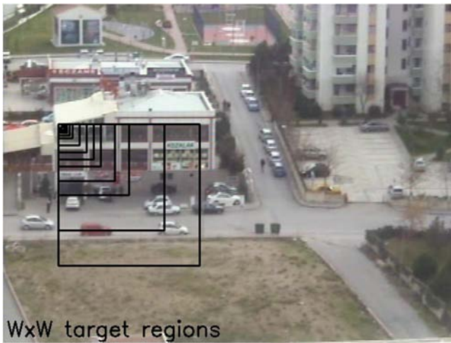
Fig. 9 The illustration of the W \times W computation region located at a reference point. The values for the target size W is selected as follows: W = \{5, 8, 10, 12, 16, 20, 30, 40, 50, 60, 80, 100, 125, 150, 200\}
