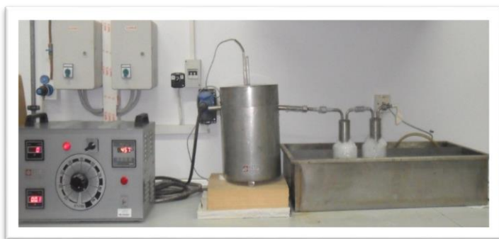
Fig. 2a. Pyrolysis system
