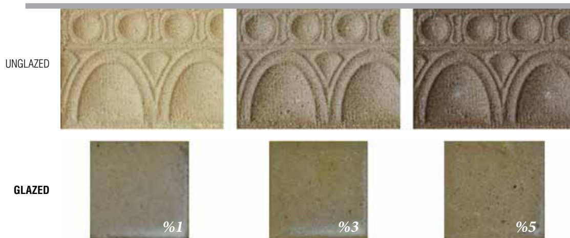
Figure 4. Firing colors of unglazed and transparent glazed of MnO added bodies at 1200°C.
