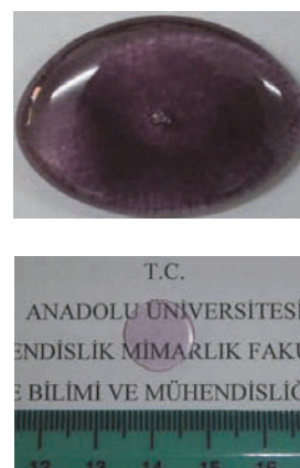
Figure 2. Thinned and polished glass sample (below) obtained from a big piece (above).
