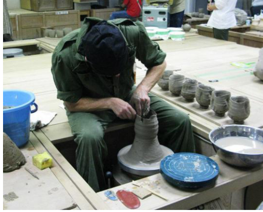
Picture 15: Electric Wheel Used in Japan and Special Working Area For Throwing.
