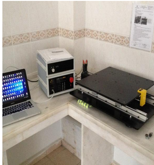
Fig. 2: Shaking table test device.
